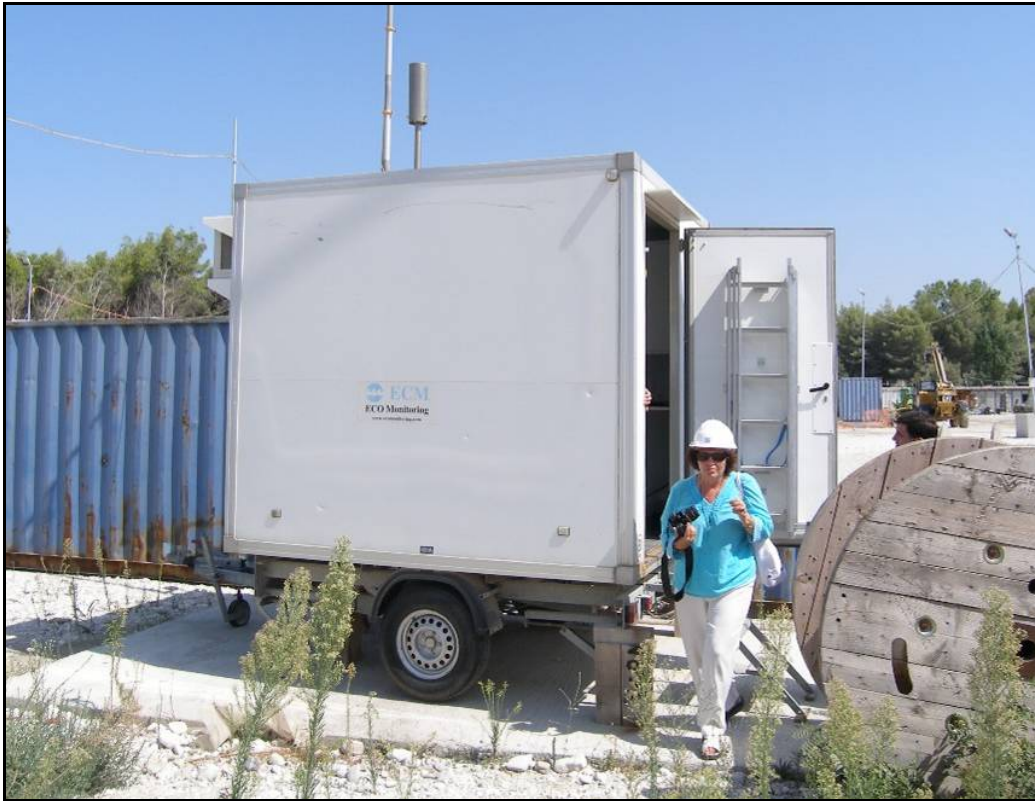
Photo 6. Mobile air monitoring station; data used to calibrate modeling
