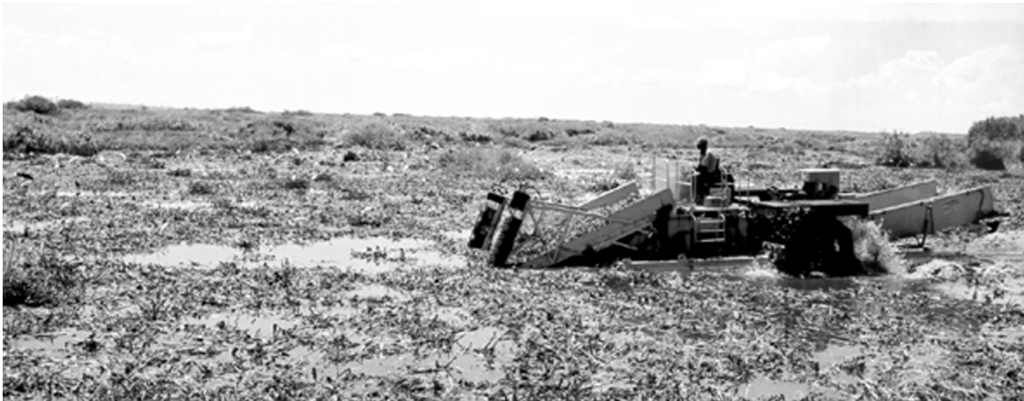
Aquatic plant shredder at work in the Nyanza Gulf where harvesting and dumping is taking place
