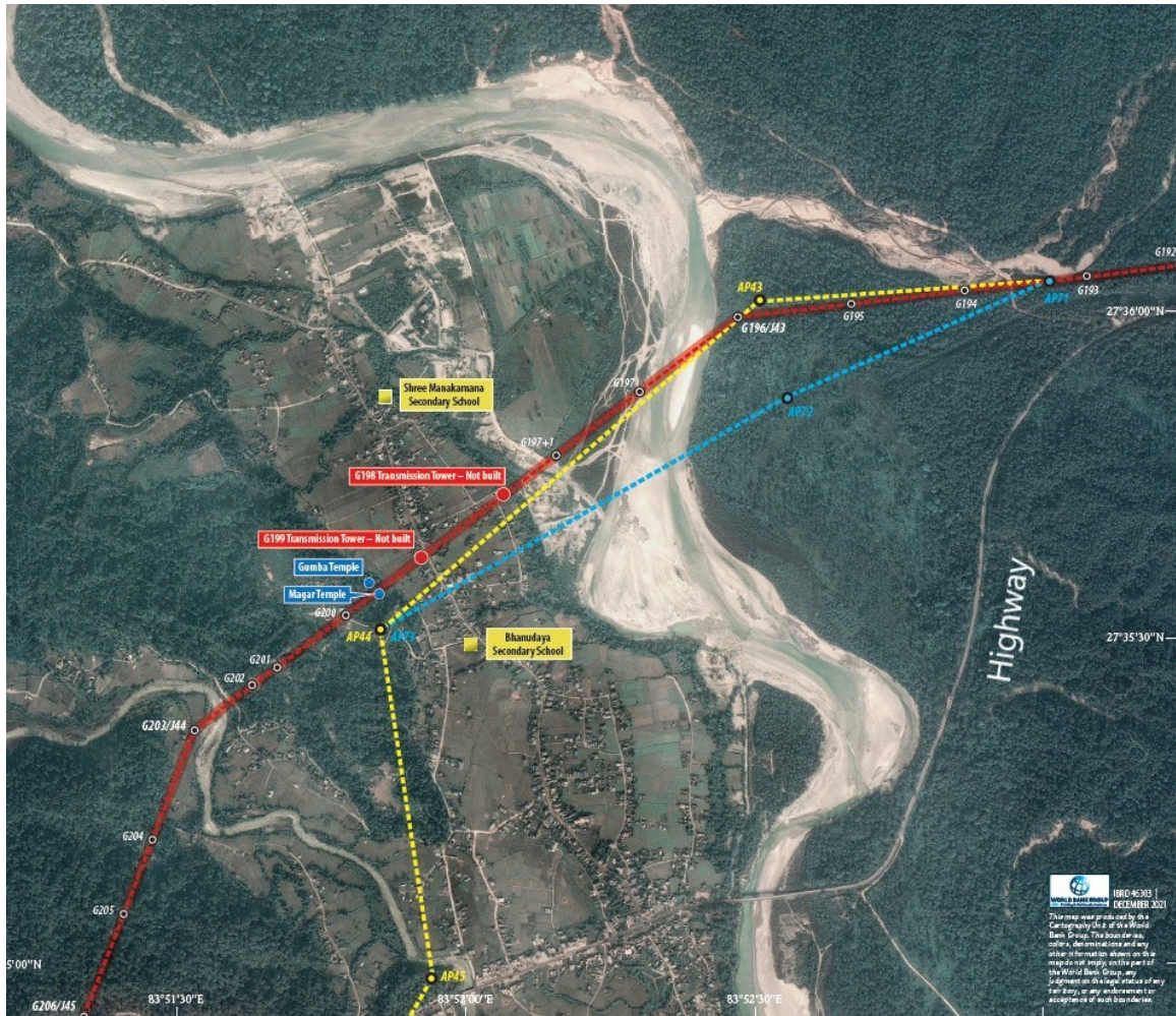
Map 2. The routing of the transmission line according to the surveys. (1998 survey - blue line; 2004 survey – yellow line; and final 2012 survey - red line)
