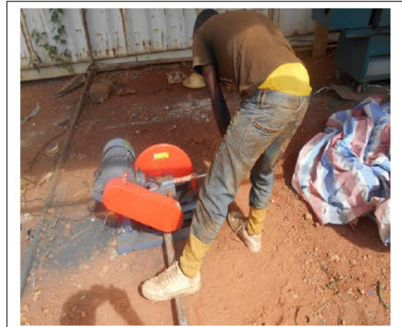
Wearing canvass in an area full of half pieces of iron. Industrial Safety at its worse.
